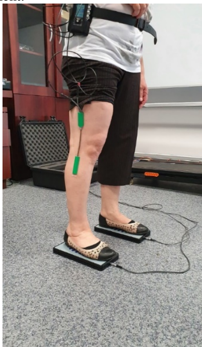
Figure 1. Placement of the electrogoniometers on the knee joint.
