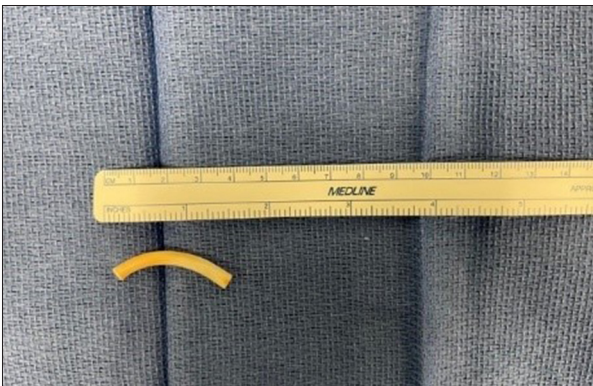
Figure 3. Cannula of the fractured tracheostomy tube after removal.
