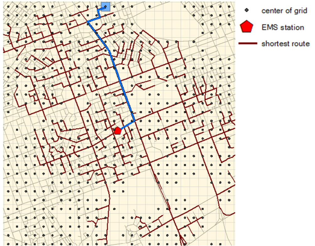
Fig 3. Illustration of per-grid evaluation of k-minute coverage using the shortest-time route.
