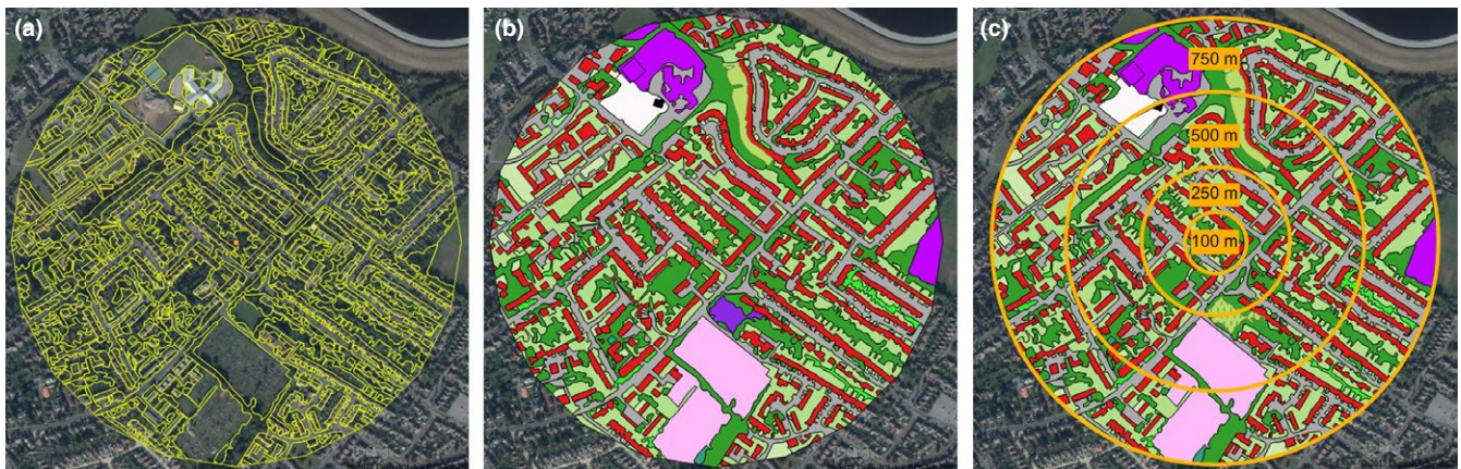
FIGURE 3 Illustration of the steps involved in manually generating a land cover map for a 750 m radius around a study site in QGIS, using an example site in the suburban region to the southwest of London, UK. (a) The first step involves drawing polygons around each land cover patch at a set scale (1:5,000 m in agricultural areas or 1:2,500 m in built-up areas) to split the data layer into a series of features representing each patch. (b) Each patch is visually classified to one of 80 land cover classes; for color legend, see Appendix S1. (c) The buffer is clipped to multiple radii representing different spatial scales at which the study taxon may interact with the surrounding land based on ecology of the organism
