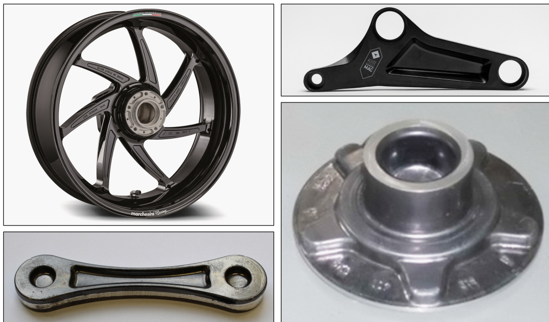
Figure 1. Various Mg forged parts, showing (u.l.) a motorbike rim produced by Brembo S.p.A. under Marchesini trademark, (u.r.) a bike suspension link made by ALLITE® Inc., (b.l.) laboratory scale piston rod forged by Light Metals Technologies Ranshofen and (b.r.) a wheel hub produced by Institut für Metallformung, University Freiberg. Reproduced with the kind permission of: Brembo S.p.A., ALLITE® Inc., Light Metals Technologies Ranshofen and TU Bergakademie Freiberg.
