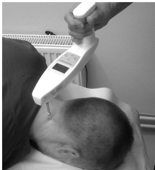
Figure 1. Measurement of the mechanical properties of splenius capitis using the Myoton.
