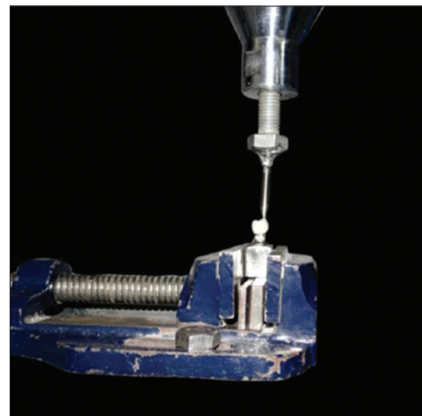
Figure 8: Specimen on universal testing machine
