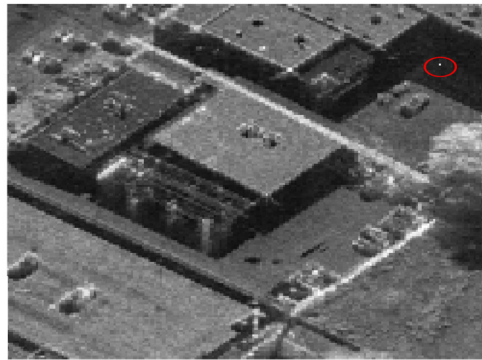
Figure 11. Focused SAR image with 0.3 m resolution for simulation.
