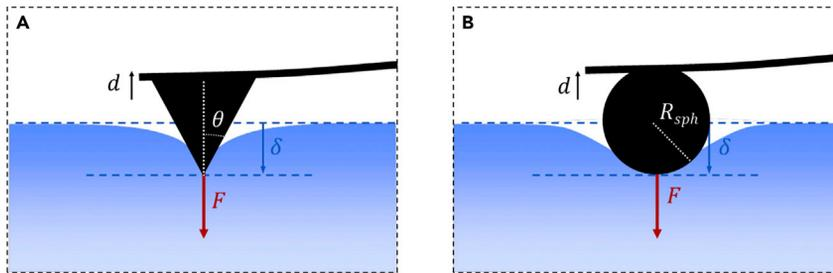
**Figure 2. Four-sided pyramidal and spherical tips.**
