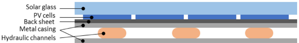
Fig. 9. Principle section schema of the PVT collector used in the experiment
