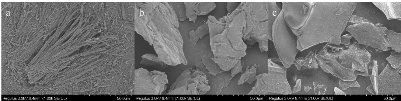
Figure 1. Microscopic morphology of sialic acid (a), chitosan (b), and 5 w/% sialic acid and 2 w/% chitosan complex (c).
