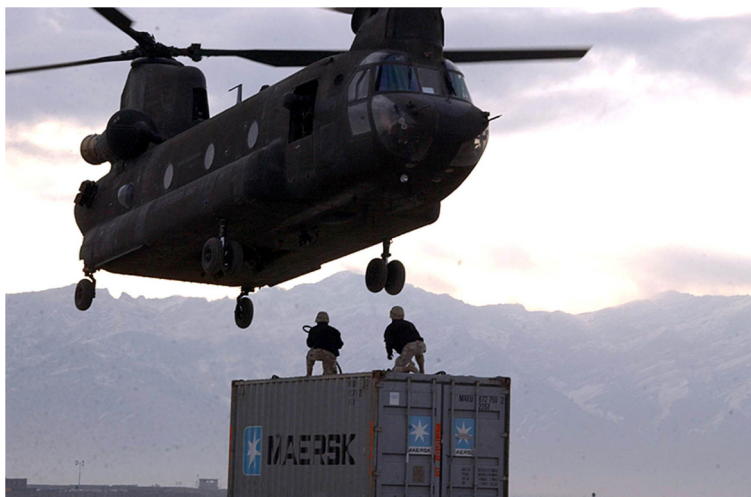
Figure 3 Chinook transport helicopter—payload 12,000 kg; range 1,100 km.
