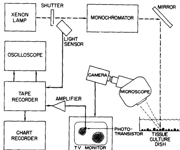
FIGURE 1. Schematic diagram of the apparatus for irradiation and recording. The heavy dashed lines represent the light path, and the heavy solid lines represent electrical wiring. Lenses have been omitted for clarity.
