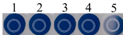
Figure 2. Five repeated BB spots. The fifth spot shows a light reflection area caused by a non-optimal cell geometry. The white circles indicated the color sampling area (120 pixels).
