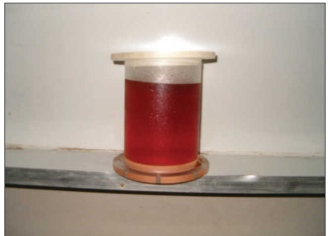
Figure 2: The plastic drink bottle modified as a gel container filled with unirradiated gel
