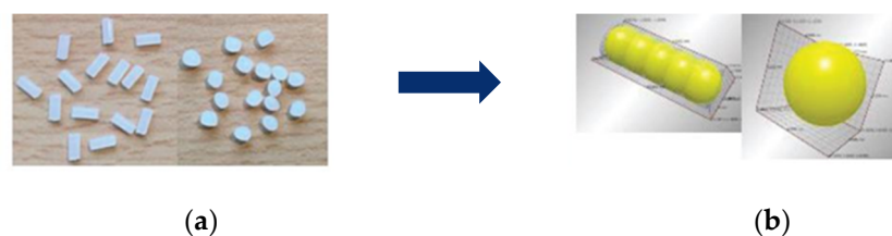
Figure 6. Transfer of the (a) real granule shape into (b) 3D simulation adapted with permission from [24]. 2021 Trippe.
