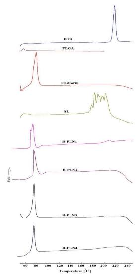
**Figure 1.** Comparative DSC thermograms of BTB, PLGA, stearin, SL and formulated lipid-polymer nanoparticles (B-PLN1 to B-PLN4).
