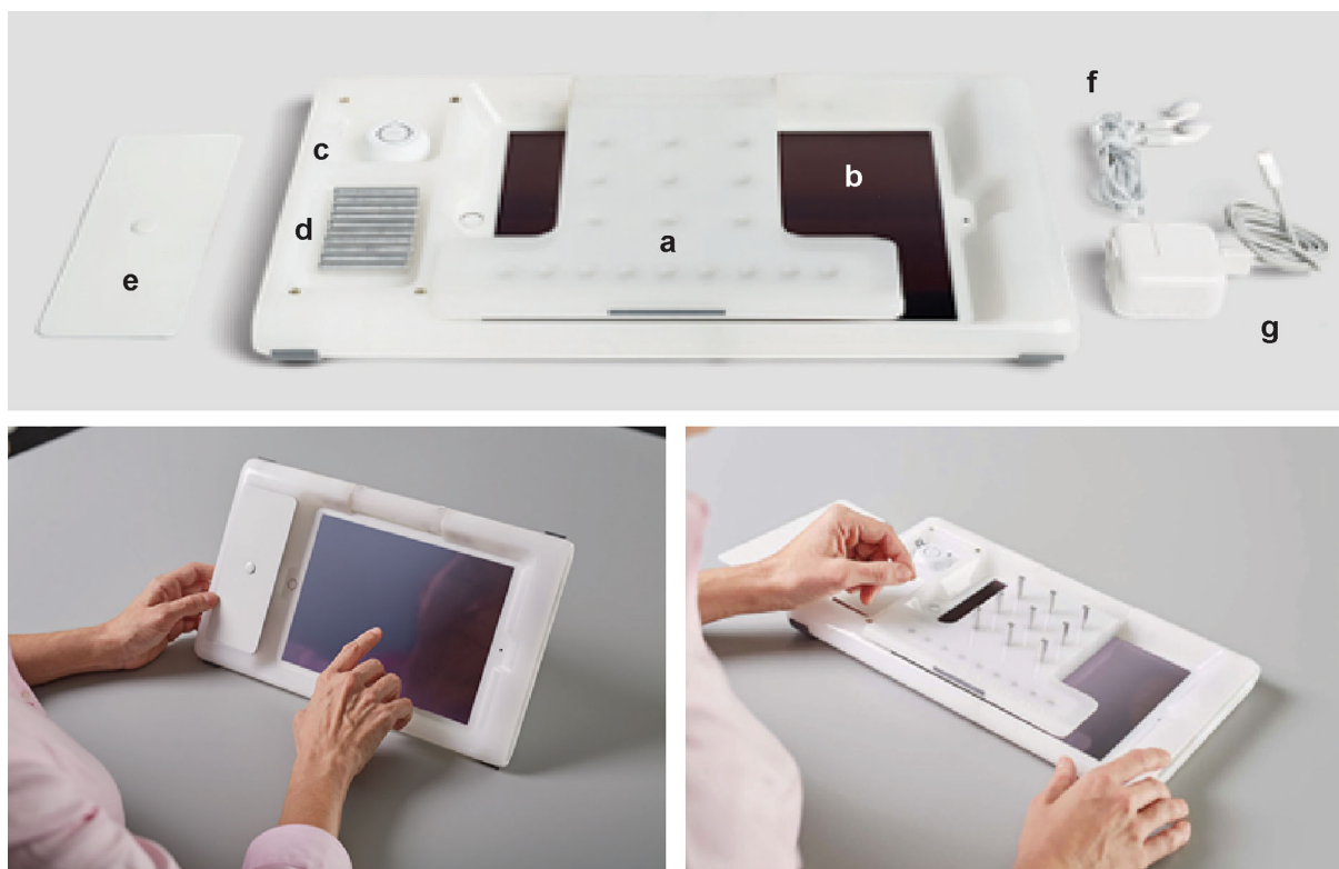
Fig. 1 MSPT assessment tool. Upper panel iPad Air® 2 contained within the hardware case, with grid overlay that also functions as a kickstand ( a ), shown over the screen ( b ). ( c ) Bluetooth remote for walking speed test; ( d ) aluminum pegs for manual dexterity test; ( e ) magnetized cover for ( c ) and ( d ); ( f ) headphones for audio instructions;
