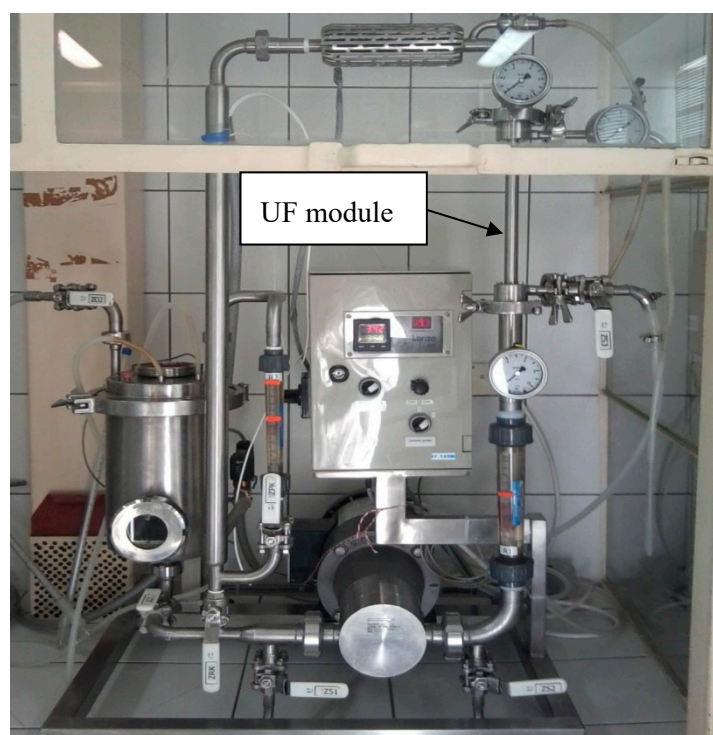
Figure 1. The photo of experimental ultrafiltration (UF) pilot-scale set-up.
