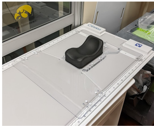
Figure 6. Custom acrylic baseplate for head-and-shoulder mask fixation and indexing.
