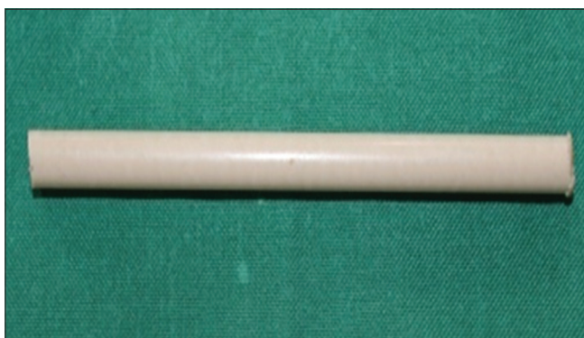
Figure 1: Poly-ether-ether-ketone ingot before milling
