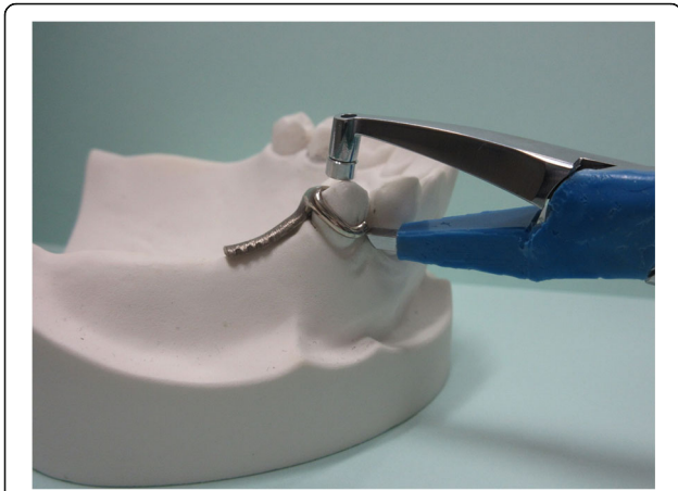
Fig. 4 The measurement situation of the small-sized retentive force measurement device
