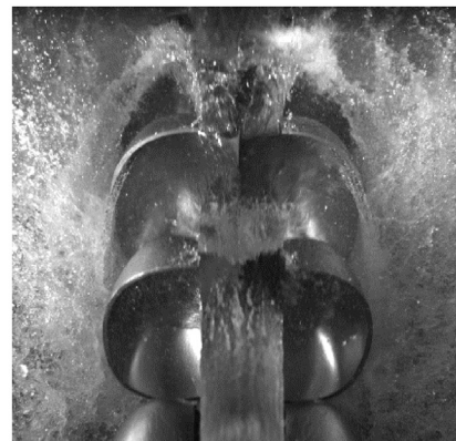
Figure 4. Flow field in a Pelton casing (a) (photo courtesy of Sean Petley, CFD simulation) and focus on the jet (photo courtesy of Bjorn Winther Solemslie).
