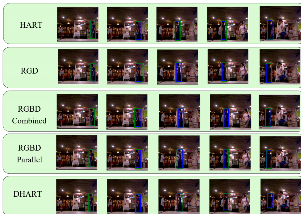
Figure 5. The object tracking model results with the Princeton dataset [4] (blue box—bounding box, green box—attention area): RGB, RGD, RGBD-combined, RGBD-parallel, and depth methods, from top to bottom, respectively. Each method successfully detected the target and tracked it. However, by using depth, the predicted bounding box was tighter.
