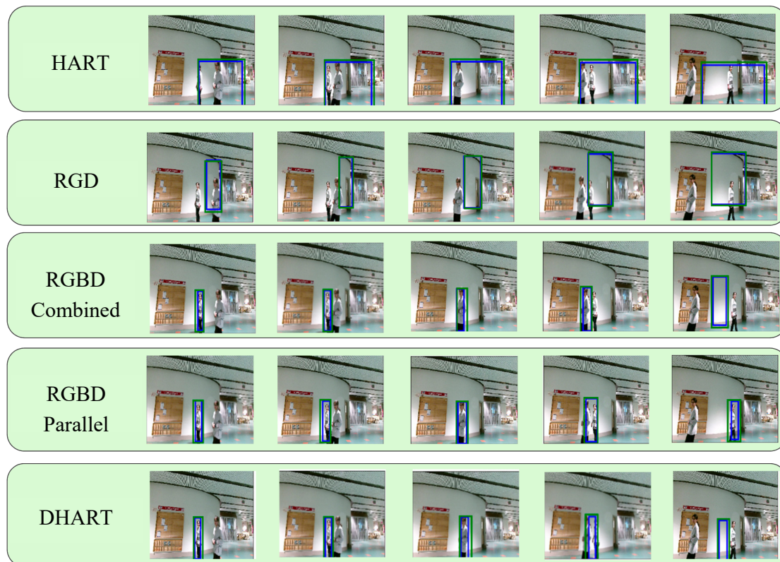
Figure 6. The object tracking model results (blue box—bounding box, green box—attention area): RGB, RGD, RGBD-combined, RGBD-parallel, and depth methods, respectively, from top to bottom. As can be seen, the color of the target, the background, and the occlusion are similar, and hence the HART algorithm was not successful tracking the target; however, the RGBD parallel model could track the target using extra depth features. Additionally, having only depth information performs better compared to having only RGB data.
