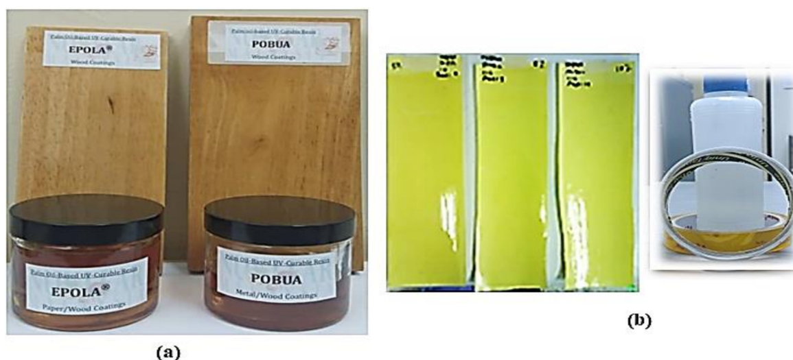
Figure 10. Radiation-curable of palm oil-based products with UV curing. (a) Acrylated and polyurethane resins for wood coating; (b) Polyurethane resins for PSA. Source: Unpublished data.
