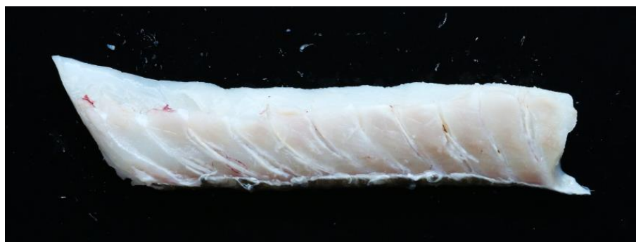
Figure 13. Example of a cod fillet treated with a 1 MHz transducer at a 45 mm distance, with continuous treatment along the row of bones at a speed of 1 mm/s. The fillet was cut along the row of bones to visualize the treatment effect. Note that some bones have become detached from the muscle, and that some have been “burned”, resulting in a brown color. The image represents a “best case” with regard to the treatment effect, and is not representative of all fillets treated.
