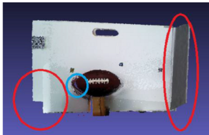
Figure 9. Registered point cloud with elastic fusion adjustment.
