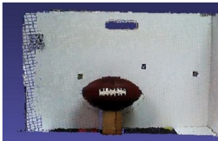
Figure 10. Registered point cloud with ICP adjustment, using VO result as the first guess.
