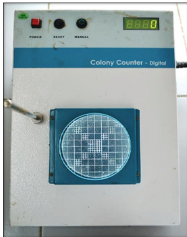
Figure 1: Digital colony counting device
