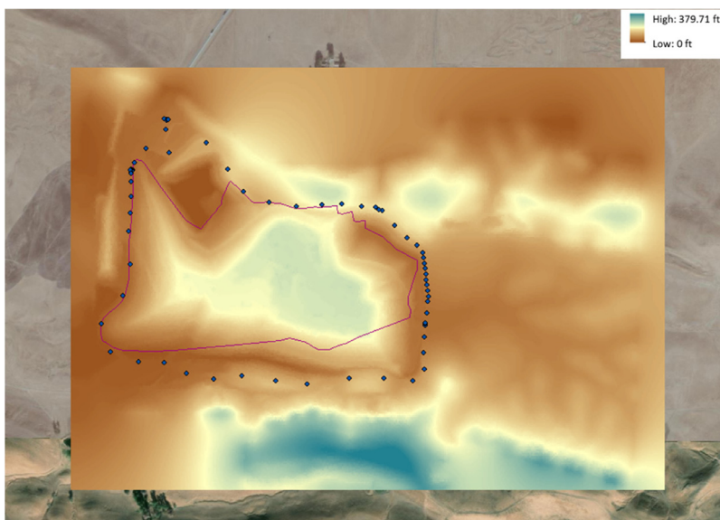
Fig. 6. Raster elevation dataset of Potrero Hills Landfill (z-scale in feet). Warm and cool colors indicate low and high elevations, respectively. The historical waste placement boundary is purple and the downwind monitoring locations with blue diamonds.
