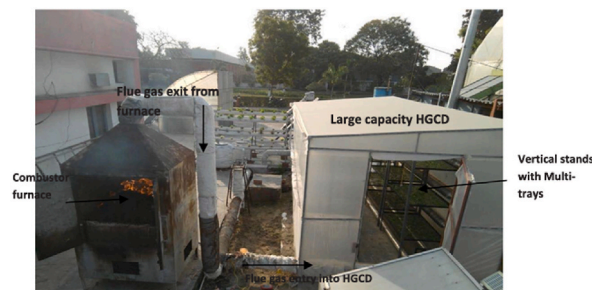
Fig. 5. Pictorial view of solar-cum-biomass hybrid greenhouse crop dryer.
