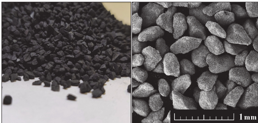
Figure 2. An example of a commercial granulate used for the deposition of thin-film superconducting tapes; photograph of GdBCO granulate (left), SEM micrograph of GdBCO granulate (right).
