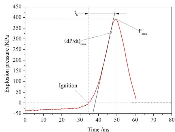
Figure 4. Typical pressure profile as a function of time during mixture explosion.
