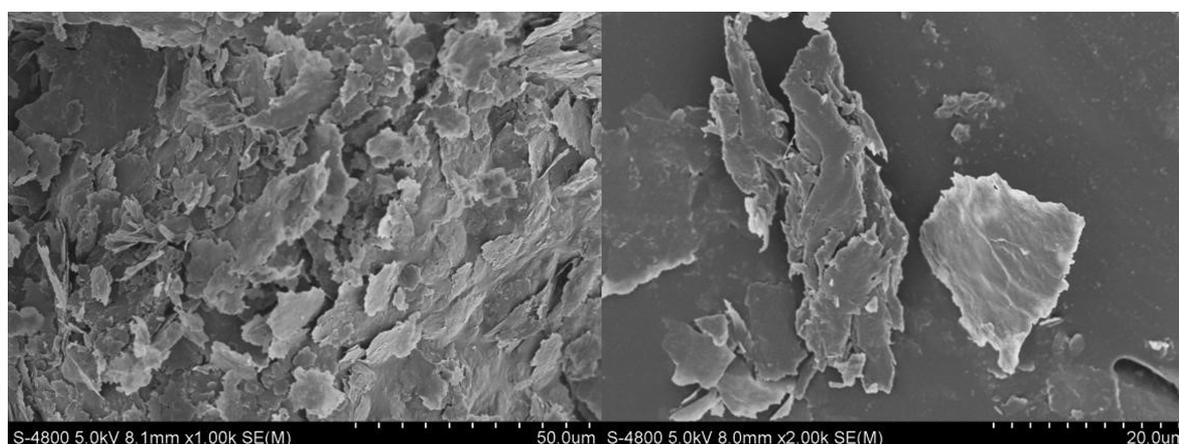
Figure 3. Scanning electron microscopy images of Al powders.
