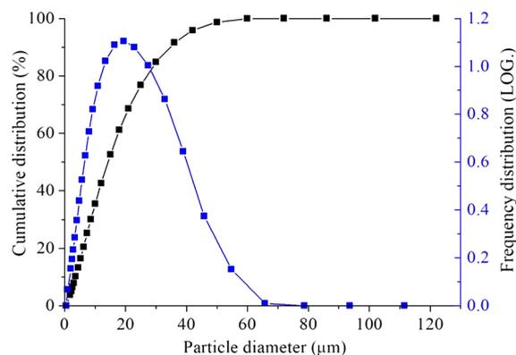
Figure 2. Particle diameter distribution of Al.
