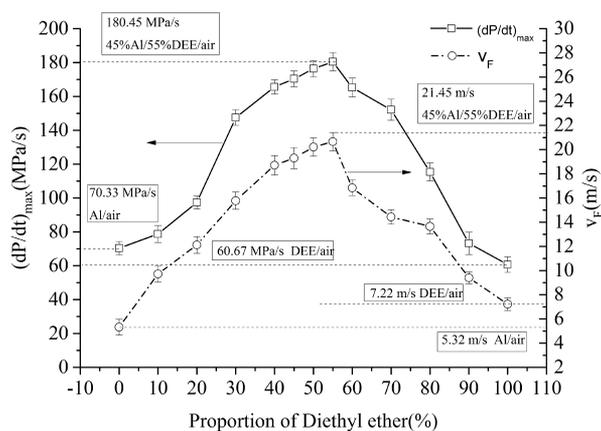
Figure 10.  $(dP/dt)_{\max}$  and flame propagation speed vs flame propagation speed.
