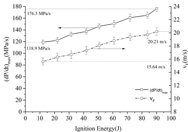
Figure 8.  $(dP/dt)_{\max}$  and flame propagation speed vs ignition energy.
