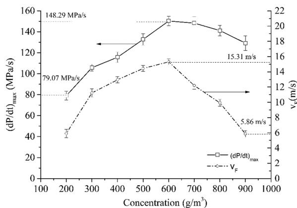
Figure 6.  $(dP/dt)_{\max}$  and flame propagation speed vs concentration.
