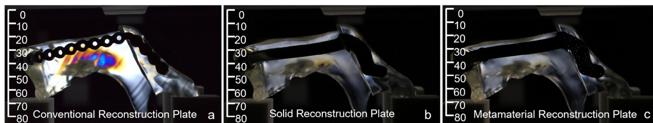
Figure 3. Original photos of unloaded samples with size annotation in mm. a) the manually contoured conventional implant shows substantial stress concentrations within the whole interior of the mandibular segments, probably induced by the manual bending, b) the solid patient-specific implant shows close-to-zero initial stresses, c) the metamaterial patient-specific implant shows close-to-zero initial stresses.
