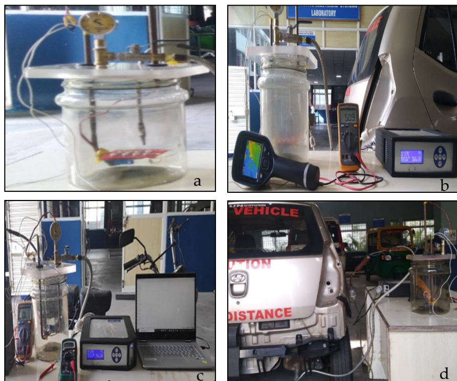
Figure 3. Experimental set-up for real-time sensor testing. (a) Sensor arrangement inside chamber with an exhaust gas analyser and a commercial CO sensor MQ-7. (b) Gas chamber with sensor arrangement connected to the measurement setup using external lead. (c) Data collection from chamber by the data acquisition system, continuously recording the values. (d) Test-vehicle engine connected to the inlet of the chamber.
