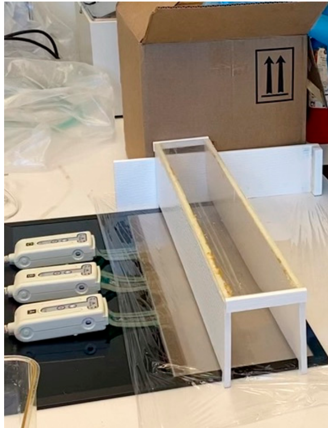
Figure 8. The gait testing unit comprising the Tekscan pressure sensor mat (black) that was modified to include a tinted Plexiglas tunnel (width: 17.0 cm; height: 17.0 cm; length: 44.7 cm) for the purpose of guiding the rats across the mat and into the goal box.
