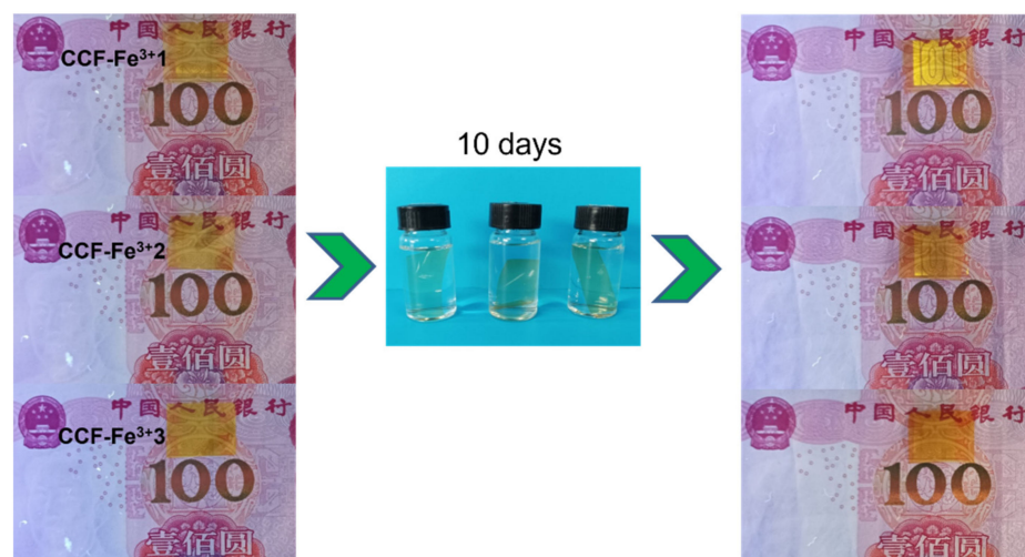
Figure 9. Effect of soaking in water (pH = 6.8) for 10 days on the UV blocking performance of CCF-Fe 3+ films.
