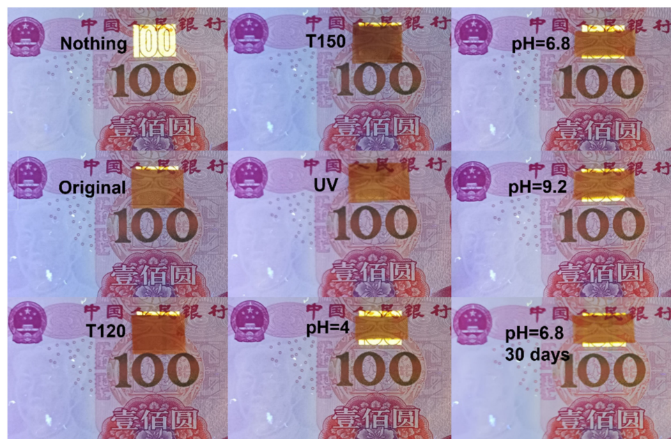
Figure 8. Paper money was shielded by M(Fe)CCF1 treated under different conditions, then exposed to UV light.
