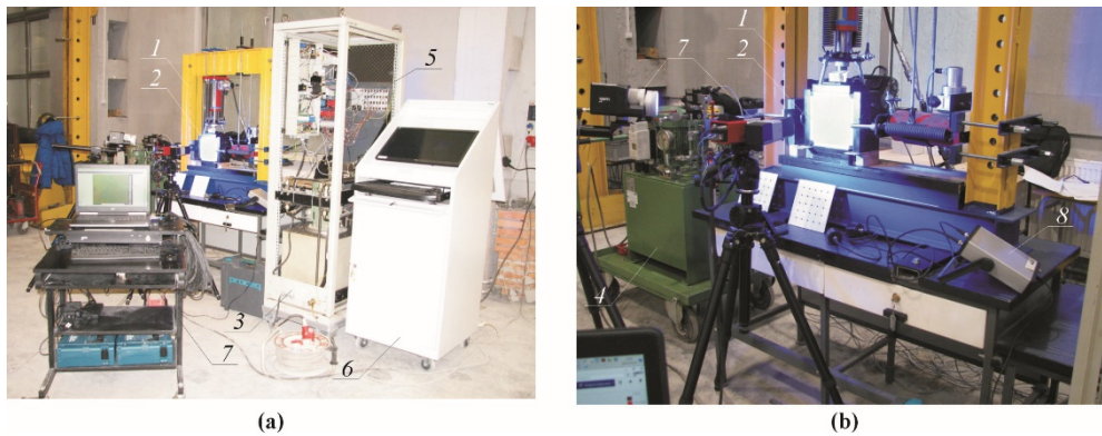
Figure 5. View of the test stand in operation: (a) overall view, (b) specimen view; 1—the test stand with the fixed actuators; 2—a test element; 3—the hydraulic system ‘A’; 4—the hydraulic system ‘B’; 5—the measurement and control interface; 6—IT system; 7—cameras of the ARAMIS 6M system; 8—PUNDIT LAB+ instrument.
