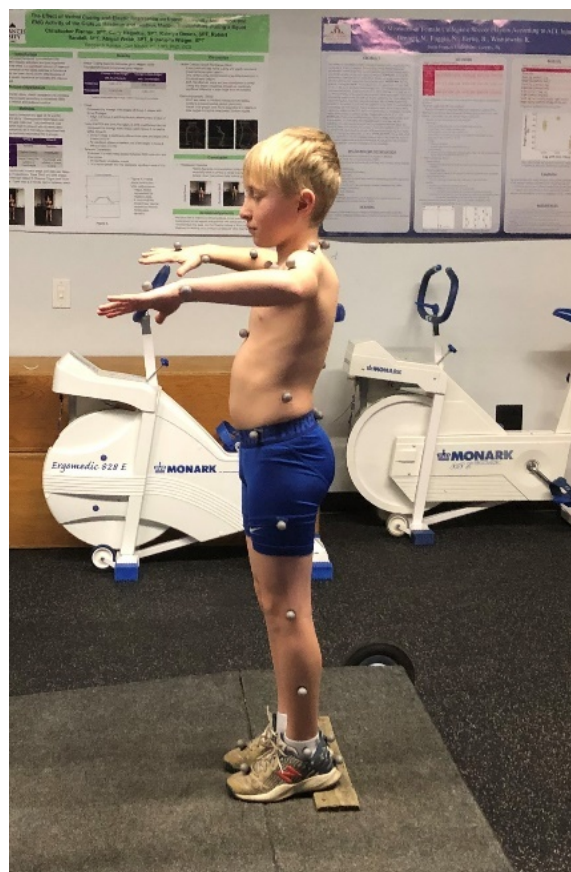
Figure 1. Reflective marker placement for 3-dimensional motion analysis during pitching trials.
