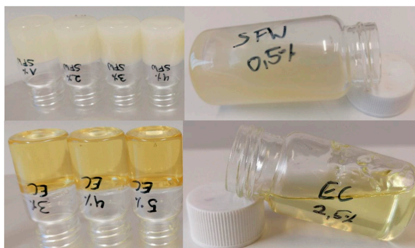
Figure 1. Upside-down test to determine critical structuring composition. After stabilization (48 h, 5 °C), sample vials with different compositions (1 to 10% (w/w) in 1% steps) are turned upside down. Stable composition left, instable composition at intermediate composition right. Top row sunflower wax in canola oil (0.5%); bottom ethylcellulose (100) in canola oil (2.5%) [66].
