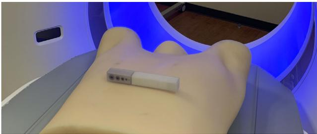
**Fig. 5.** Simulated use of calibration mini-phantom in clinical CT. Demonstration photograph of the calibration mini-lung-phantom placed on top of an anthropomorphic thorax phantom, as an example placement of the mini-lung-phantom on the patient chest in clinical chest CT.
