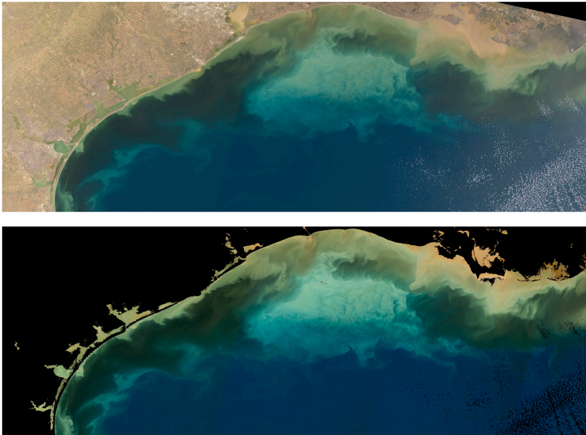
Figure 10. OLCI (Sentinel 3A) true color reconstruction 24 January 19, 16:29 UTC, central and northwestern Gulf of Mexico (top \rho_s ; bottom \rho_w ). Note there is some atmospheric correction (aerosol) failure in the bottom image.
