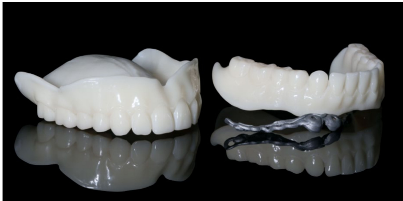
Figure 10. Additively manufactured try-in dentures for the upper and lower jaw and selectively laser sintered (SLS) alloy framework.
