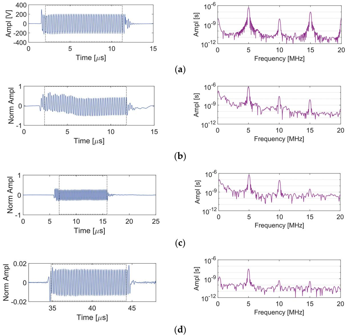
**Figure 5.** A-scans and frequency spectra for 5 MHz toneburst excitation at the 75% output level: (a) Point A, (b) Point B, (c) Point C, and (d) Point D.
