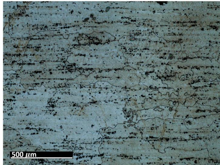
**Figure 2.** Optical microscope (Zeiss SmartZoom) image of polished and etched (Kroll's reagent) aluminum block surface. Pancake-type grains and a distribution of fine precipitates are apparent.
