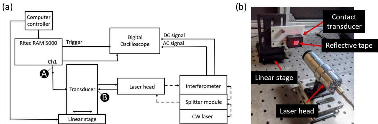
**Figure 1.** Test setup for measurement of system nonlinearity: (a) Block diagram where solid and dashed lines represent electrical cables and optical fibers respectively, (b) Photograph of the laser head illuminating reflective tape on the transducer surface.
