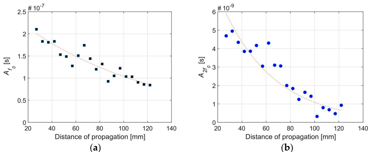
Figure 11. Sample attenuation curves for (a) primary (2 MHz) and (b) secondary (4 MHz) waves from Sample 3.
