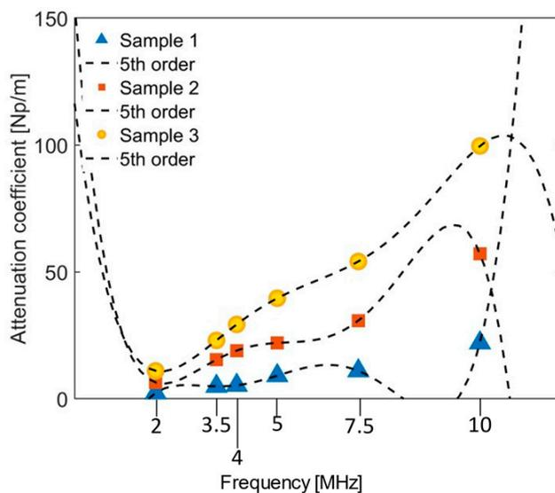
Figure 12. Frequency dependence of the attenuation coefficients for Rayleigh waves on aluminum block.
