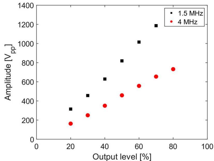
**Figure 4.** Amplitude of toneburst signal sent to the transducer as a function of amplifier output level for center frequencies of 1.5 and 4.0 MHz.
