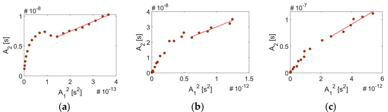
**Figure 6.** Linear regression to determine the relative nonlinearity parameter for the sensing system given a 5 MHz signal: (a)  $\beta' = 16433$  at Point A, (b)  $\beta' = 16790$  at Point B, (c)  $\beta' = 17019$  at Point C.
