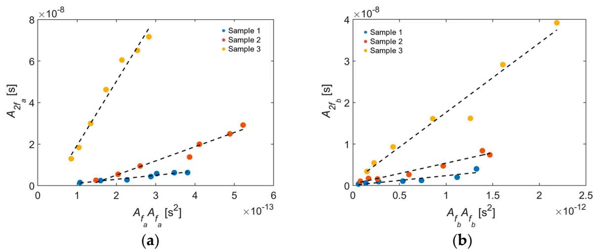
**Figure 9.** Second-order spectral amplitudes for self-interaction plotted as a function of the square of the primary frequency amplitudes for (a)  $2f_a$  and (b)  $2f_b$ .  $f_a = 1.5$  MHz and  $f_b = 4.0$  MHz.
