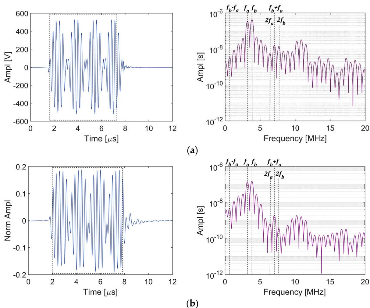
**Figure 7.** A-scan and frequency spectrum given a dual-frequency excitation ( $f_a = 3.2$  MHz and  $f_b = 3.8$  MHz) excitation at the 75% output level: (a) Point A, (b) Point B.
