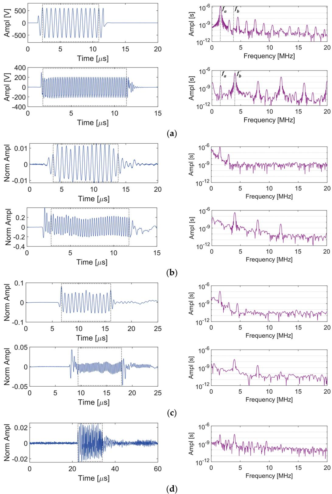
**Figure 8.** A-scan and frequency spectrum given toneburst excitations to adjacent transducers at the 75% output level: (a) Point A, (b) Point B, (c) Point C, (d) Point D.
