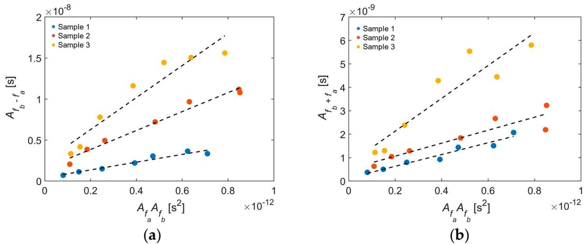
**Figure 10.** Second-order spectral amplitudes for mutual interaction plotted as a function of the product of the primary frequency amplitudes for (a)  $f_{b-a}$  and (b)  $f_{b+a}$ .  $f_a = 1.5$  MHz and  $f_b = 4.0$  MHz.
