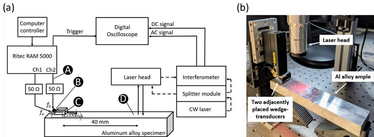
**Figure 3.** Rayleigh wave test setup: (a) Block diagram where solid and dashed lines represent electrical cables and optical fibers respectively, (b) Adjacent angle-beam transducers actuate dual-frequency Rayleigh waves, which are received by the laser head.
