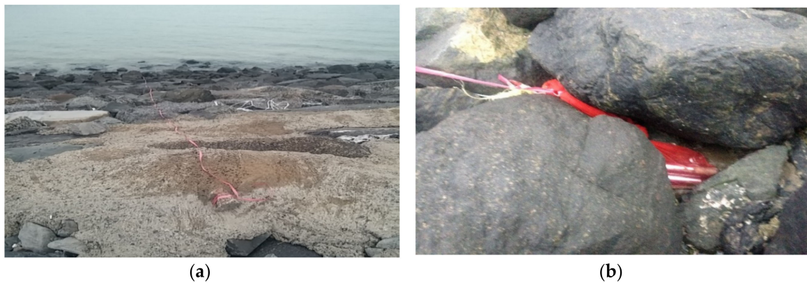
Figure 2. Sea water test of the materials for the cover of the FBG sensors: (a) during the tide; and (b) during the ebb tide.
