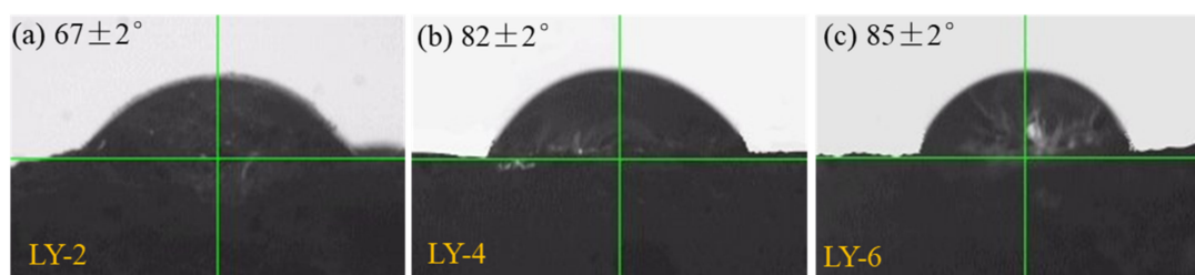
Figure 3. Contact angles of concrete at 28 days: (a) LY-2; (b) LY-4; (c) LY-6.
