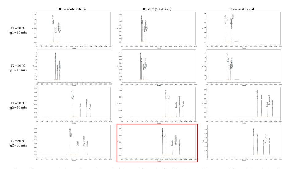
**Figure 2.** Chromatograms of reference substances aloe-emodin, rhein, emodin, chrysophanol, and physcion for the 12 input runs at 435 nm. tg1: time of gradient 1 (10 min from 1 to 99% B), tg2: time of gradient 2 (30 min from 1 to 99% B)
