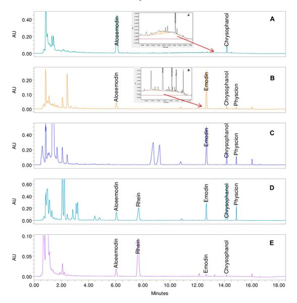
**Figure 7.** Chromatograms at 435 nm with the selected gradient 1 of the five drug samples (drug solvent ratio 100 mg:1 mL) (**A**) dried leaf juice of *Aloe barbadensis* Mill. (with detailed view: 7.5–17 min); (**B**) bark of *Rhamnus purshianus* DC. (with detailed view: 9–17 min); (**C**) bark of *Rhamnus frangula* L.; (**D**) roots of *Rheum palmatum* L.; (**E**) pods of *Cassia angustifolia.*
