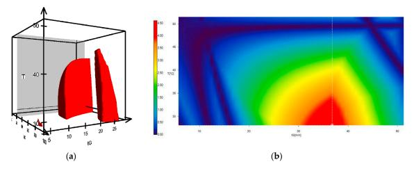
**Figure 4.** (a) Calculated resolution cube showing the working points with a resolution  $\geq 1.5$  for the critical peak pair of the 18 peaks subjected to the model. (b) Graphical view of the peak resolution in a cross section of the organic eluent acetonitrile/methanol (78:22 v/v) as a function of the temperature and gradient time. Color scale shows the predicted resolution of the critical peak pair.
