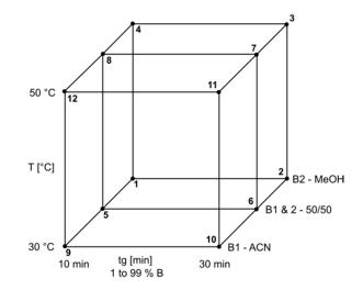
**Figure 8.** Design of experiment for the model of temperature (T), gradient time (tg), and organic modifier (B1–2). ACN: acetonitrile; MeOH: methanol; B1 and 2: mixture of both 50:50 v/v, all solvents with addition of 0.1% formic acid.
