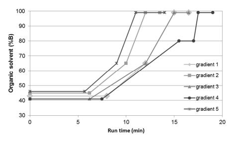
**Figure 5.** Selected gradients at working point 22% MeOH in ACN as an organic modifier and column temperature of 30  $^{\circ}$ C.
