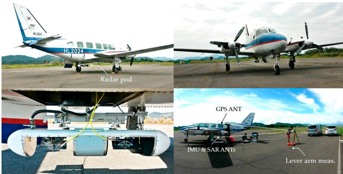
Figure 8. Overview of the airborne FMCW SAR system: radar pod was mounted at the bottom of the fuselage of PIPER PA31-350 and Tx/Rx antennas of NanoSAR-B were installed for left-looking as a default setup. The lever arm was measured with a total station, then its spatial coordinate was entered into NanoSAR-B as a system parameter and used for SAR image focusing.
