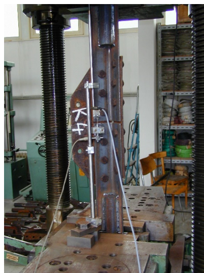
Figure 5. Test piece arrangement in the tensile testing machine.
