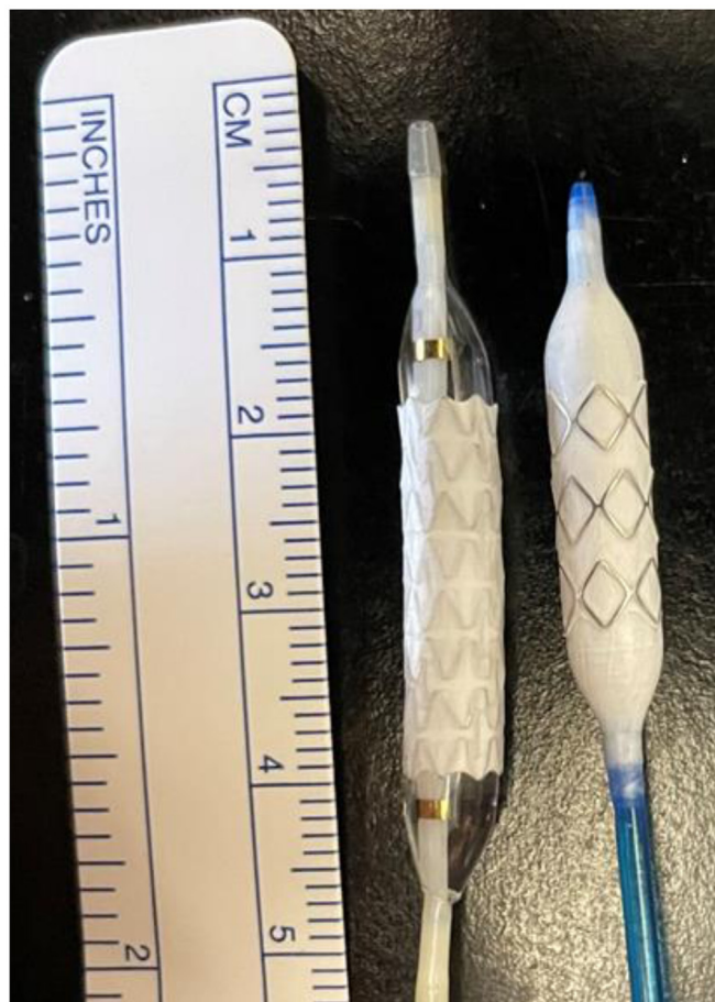
Fig 4. Comparison of Atrium iCAST (left) and Gore VBX (right) balloon-expandable covered stents after inflation with saline aligned at the distal balloon attachment point.
