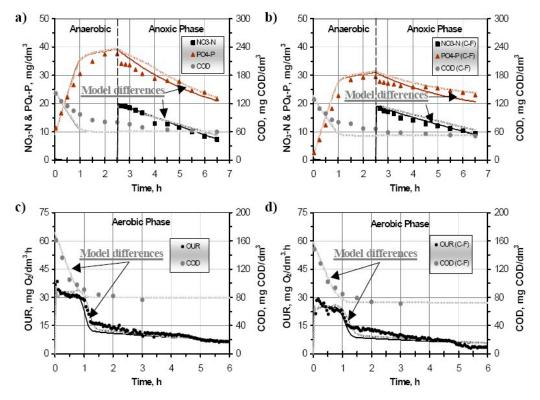
**Figure 3.** Experimental data and model predictions in the batch test treating SWW without pretreatment and after C–F. Solid lines corresponds to conventional ASM2d predictions and dashed ones to the modified ASM2d predictions. (**a**) PRR/anoxic PUR tests without pretreatment; (**b**) C–F treatment for PRR/anoxic PUR tests; (**c**) OUR tests without pretreatment; (**d**) C–F treatment for OUR tests.
