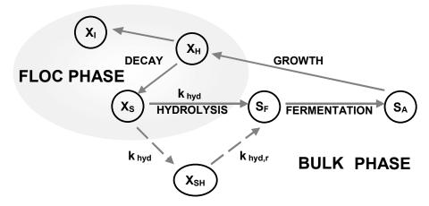
**Figure 2.** Scheme of the ASM2d, in continuous lines, and the modification proposed in the hydrolysis process, in dashed lines. X<sub>I</sub>: Inert particulate substrate; X<sub>H</sub>: Heterotrophic organisms; X<sub>S</sub>: Particulate substrate; X<sub>SH</sub>: Rapidly hydrolysable substrate; S<sub>F</sub>: Fermentable substrate; S<sub>A</sub>: Fermentation product; K<sub>hvd</sub>: First Hydrolysis stage; K<sub>hvd,r</sub>: Second Hydrolysis stage.
